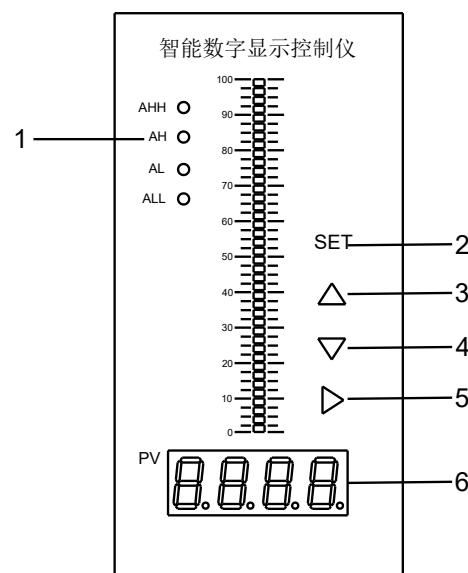
1) Indicator light AH light: The upper limit relay output; AHH light: The upper upper limit relay output
