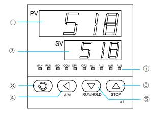
**Basic display status :** When power on, the upper display window of the instrument shows the process value (PV), and the lower window shows the set point (SV). This status is called basic display status. Symbol description was shown as following table:
