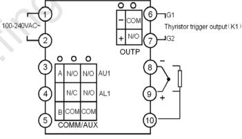
parameter bAud = 2, it can be used for AU1 or AL1 alarm output. If L1, L2, L4, G, K1, W1 or W2 is installed, it can be the auxiliary output in bidirectional (heating/refrigerating) control (Auxiliary output doesn't support analog current output); if I2 is installed and bAud = 1, then it can input on-off signal to switch SP1 and SP2 (AI-518) or switching the program status RUN / Stop (AI-518P) by connecting a switch between terminals number 3 and 5.
