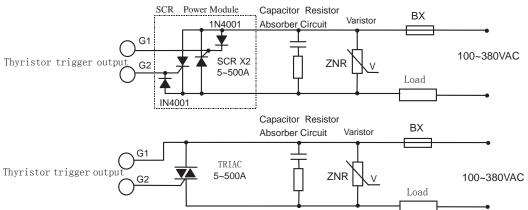
Note 1: According to the voltage and current of load, choose a suitable varistor to protect the thyristor. A resistor-capacitor circuit (RC circuit) is needed for inductance load or phase-shift trigger output.
